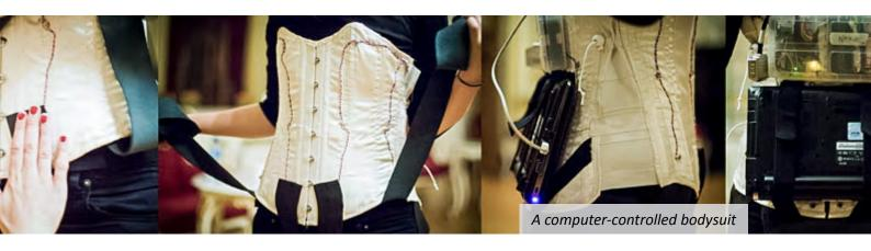
The bodysuit is a stand-alone application based on mini-pc's in combination with custom built Arduino controller-board. It is an open-source project working with the development of haptic and tactile storytelling.
